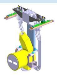
We designed the fixtures needed to precisely position the High Flux Test Module in the IFMIF-DONES test cell..
